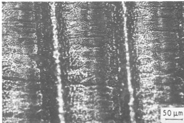
Figure 3 Plan view of copper laser-treated with 200 \text{ MW cm}^{-2} power density and three laser scans.
